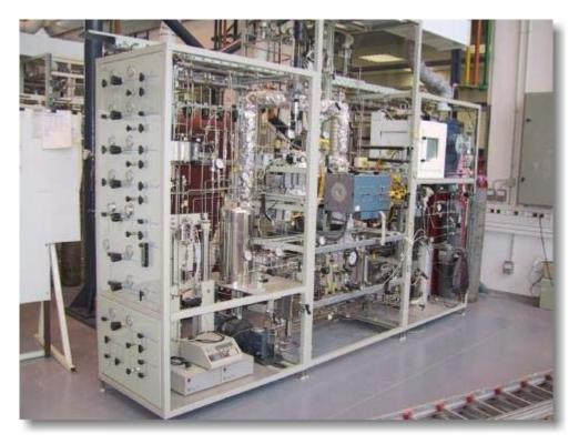
Spouted bed is a promising reactor configuration in oxidative partial oxidation process, because it combines short residence times for the gas phase along with almost perfect mixing of the solid particles, which enhances the heat transfer inside the bed. The pilot plant is constructed in modules, and can be divided into the following discrete sections:
